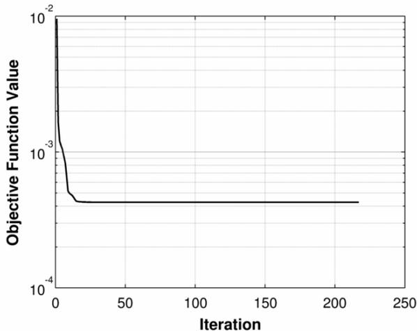
**Fig. 1.** Convexity of the mesh-based spherical deconvolution. A representative plot of the value of  $\|\mathbf{Ax}-\mathbf{b}\|_2^2 + \tau\|\mathbf{Dx}\|_p^p$  with respect to iteration for solution of a simulated  $90^\circ$  fiber crossing.
