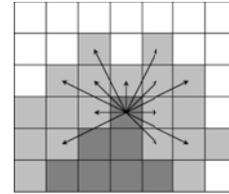
**Fig. 1.** Front evolution in fast-marching tractography. One voxel from the band under consideration (*light gray*) is accepted into the advancing front (*dark gray*) at each iteration. Arrows indicate potential transitions from one voxel on the edge of the front. A speed function dictates which transition is made.
